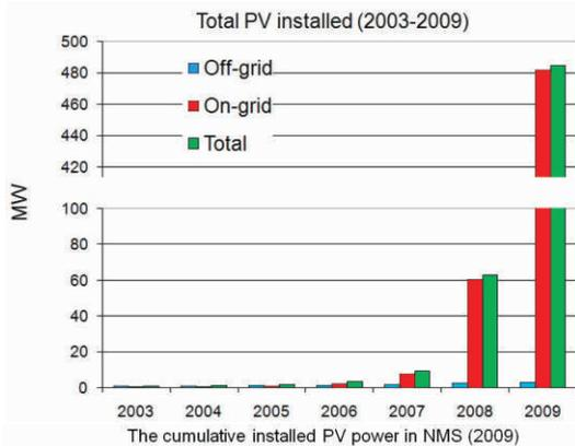
Cumulative installed PV power in NMS (2009)
