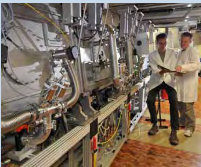
Fig. 6 - Laboratory deposition system for the preparation of amorphous and mikromorphous Silicon Thin Film devices (photo: Forschungszentrum Jülich GmbH).
