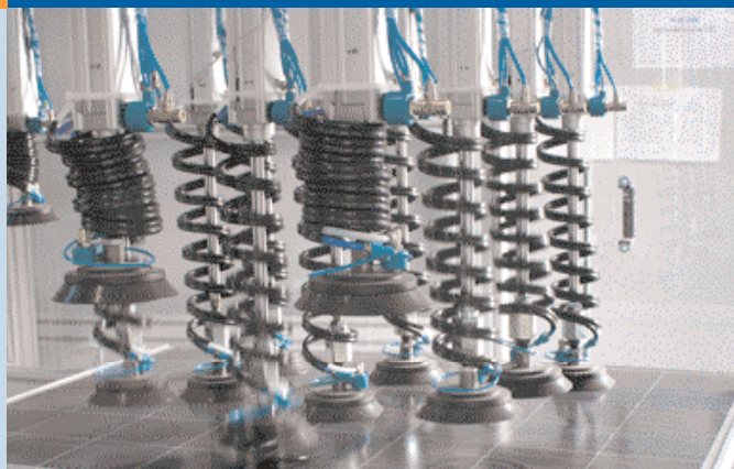
Fig. 2 - Mechanical testing for PV module certification. The University of Applied Sciences in Lugano has built a new laboratory for module testing according to IEC standards (photo ISAAC, SUPSI, Switzerland).
