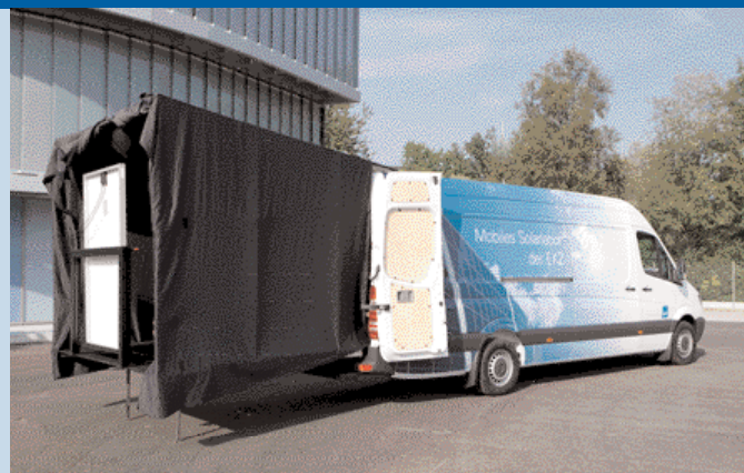
Fig. 3 - Mobile test equipment. With the support of the utility of the Canton of Zurich, the Uni-versity of Applied Sciences in Winterthur has built a mobile test unit which allows PV module testing at the site of a PV plant (photo EKZ, Zurich).
