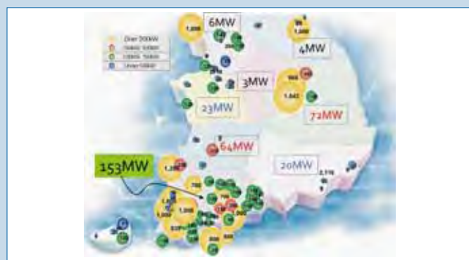
Fig. 4 - The PV power plant map in Korean Peninsula as of February, 2009. The total number of PV plant reaches to 963 and cumulative PV power generation is 287 GWh by the early of 2009.
