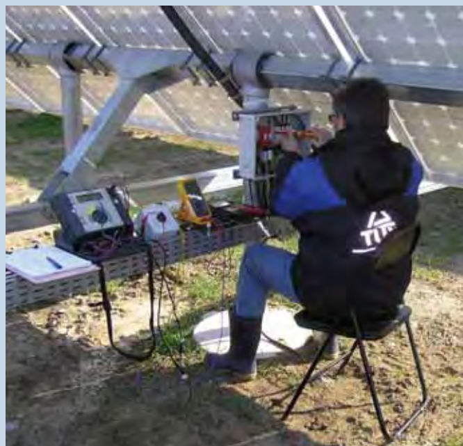
Fig. 2 - PV system performance assessment - Monitoring and inspection of PV plant in Southern Germany (photo: TÜV Rheinland).
